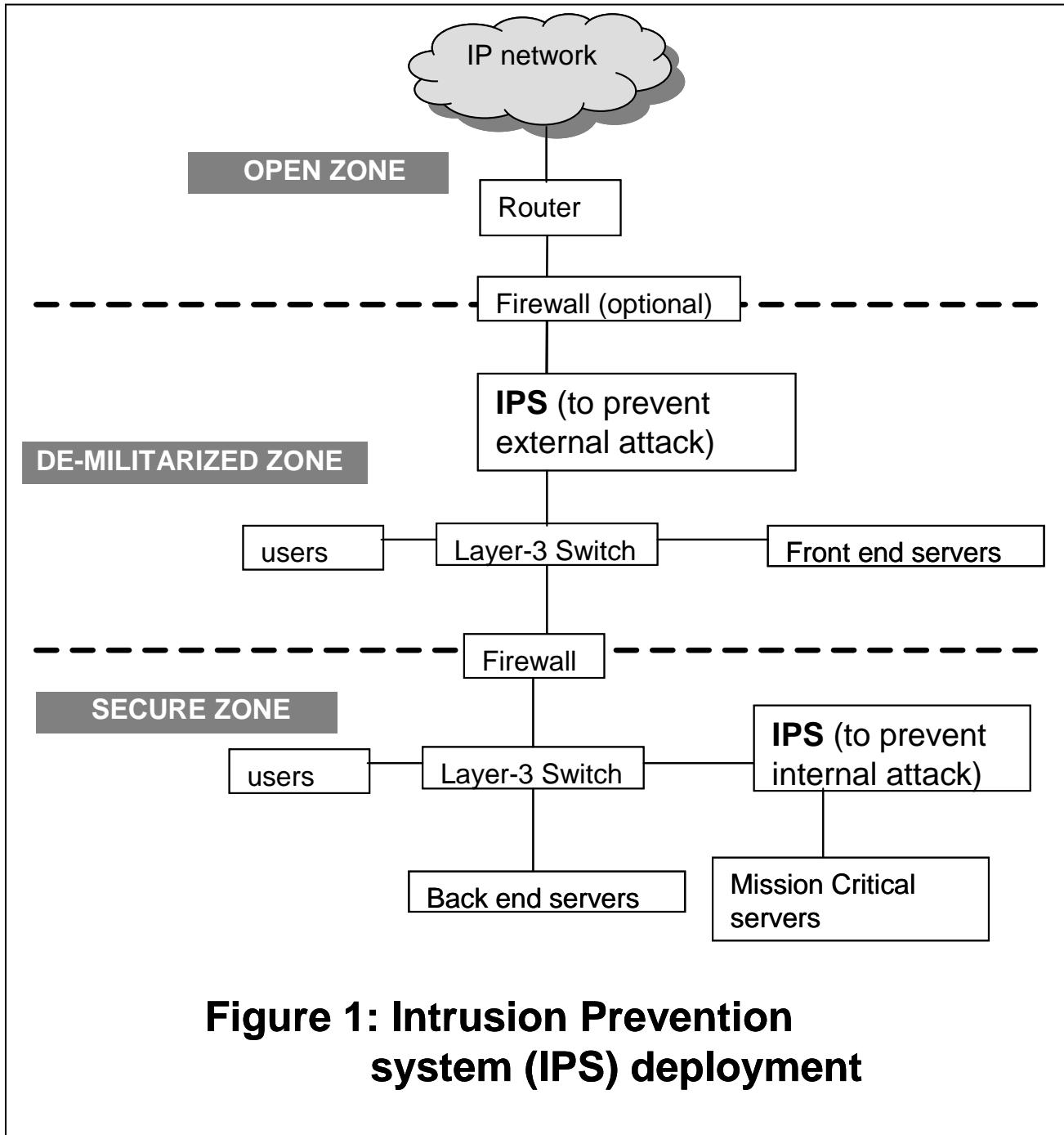
**Figure 1: Intrusion Prevention system (IPS) deployment**
